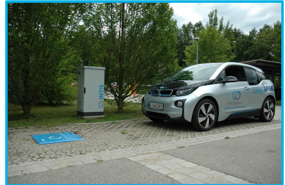
inductive charging station with retrofitted BMW-i3 (11kW)
